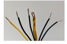
Next, we need to strip the ends of those wires. We need about 11mm (doesn't have to be perfect) of exposed wire to insert into the WAGO 221 adapter.
