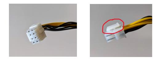
Notice that the 12V wires in this picture are yellow. Some PSUs have all black wires, so we know the 12V wires are the 4 wires closest to the lock clip (circled in red in the pictrure on the right). The 4 wires on the bottom side (from the lock clip) are ground. If your PSU 12V wires are black, you will want to mark them (perhaps with red electrical tape) before you proceed to the next step.
