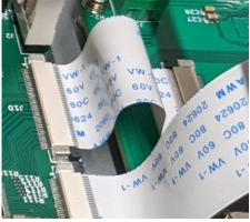
To power the **PoE Board(s)**, you must connect your VOITA Power Converter (see first picture below) to both your PSU and your first PoE Board. <u>You only need to connect the VOITA to ONE</u> PoE Board since power is shared between PoE Boards via the FFC cables.
