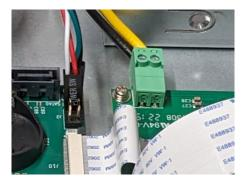
Each Interceptor Case includes four **cooling fans**, which are simple to connect to the four 3-pin fan connectors on your Interceptor Carrier Board (see pictures below).
